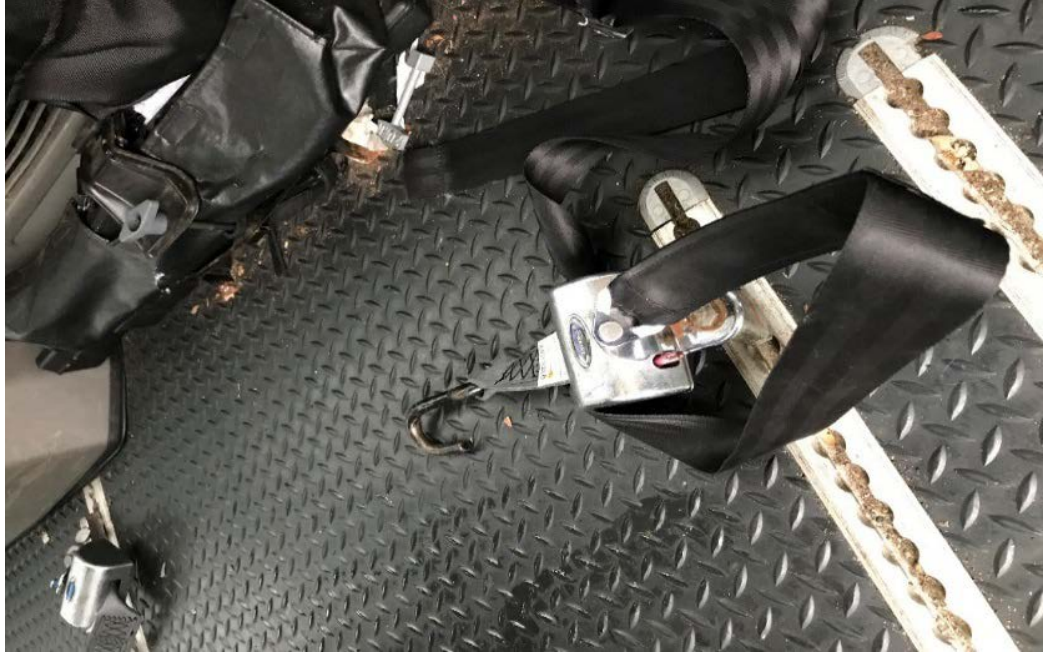
Photo of wheelchair securement equipment in the Boght Road IRA wheelchair van
